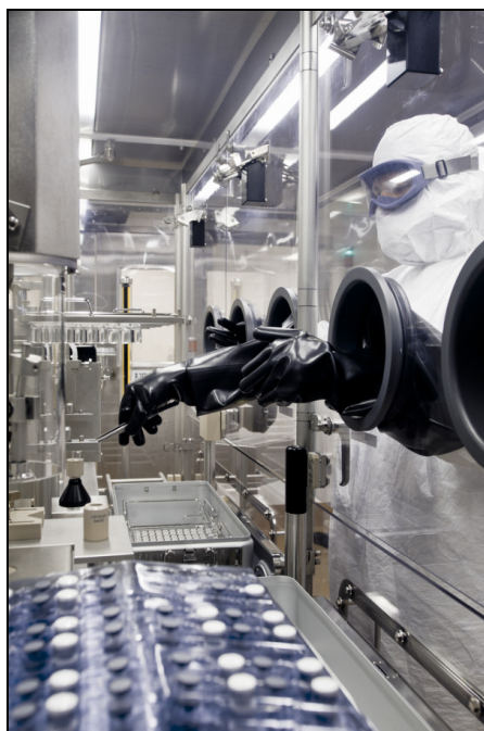
Picture caption: Semi-automated filler at Vetter's Chicago facility: Vial filling.
