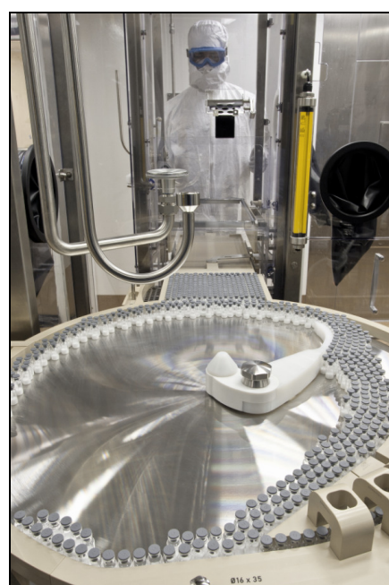
Picture caption: Fully automated vial filler at Vetter's Chicago facility: Lyophilized vials are prepared for capping.
